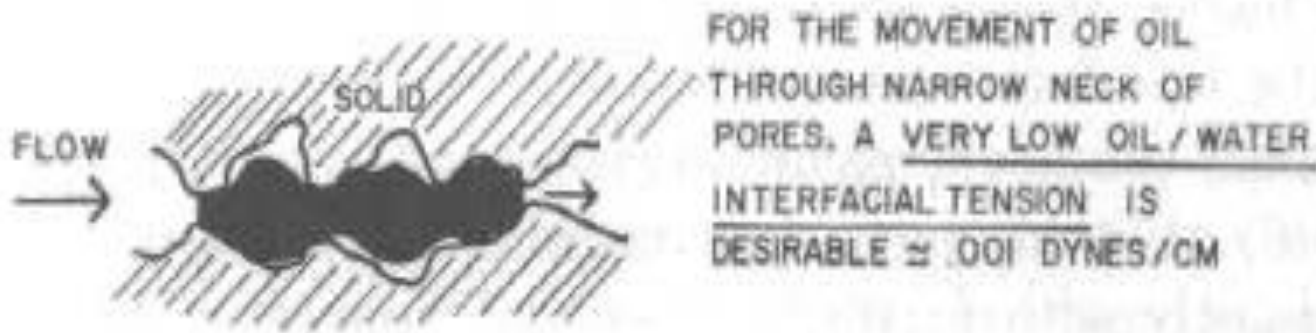
Fig. 10-3. Schematic diagram of the role of interfacial tension in surfactant flooding
