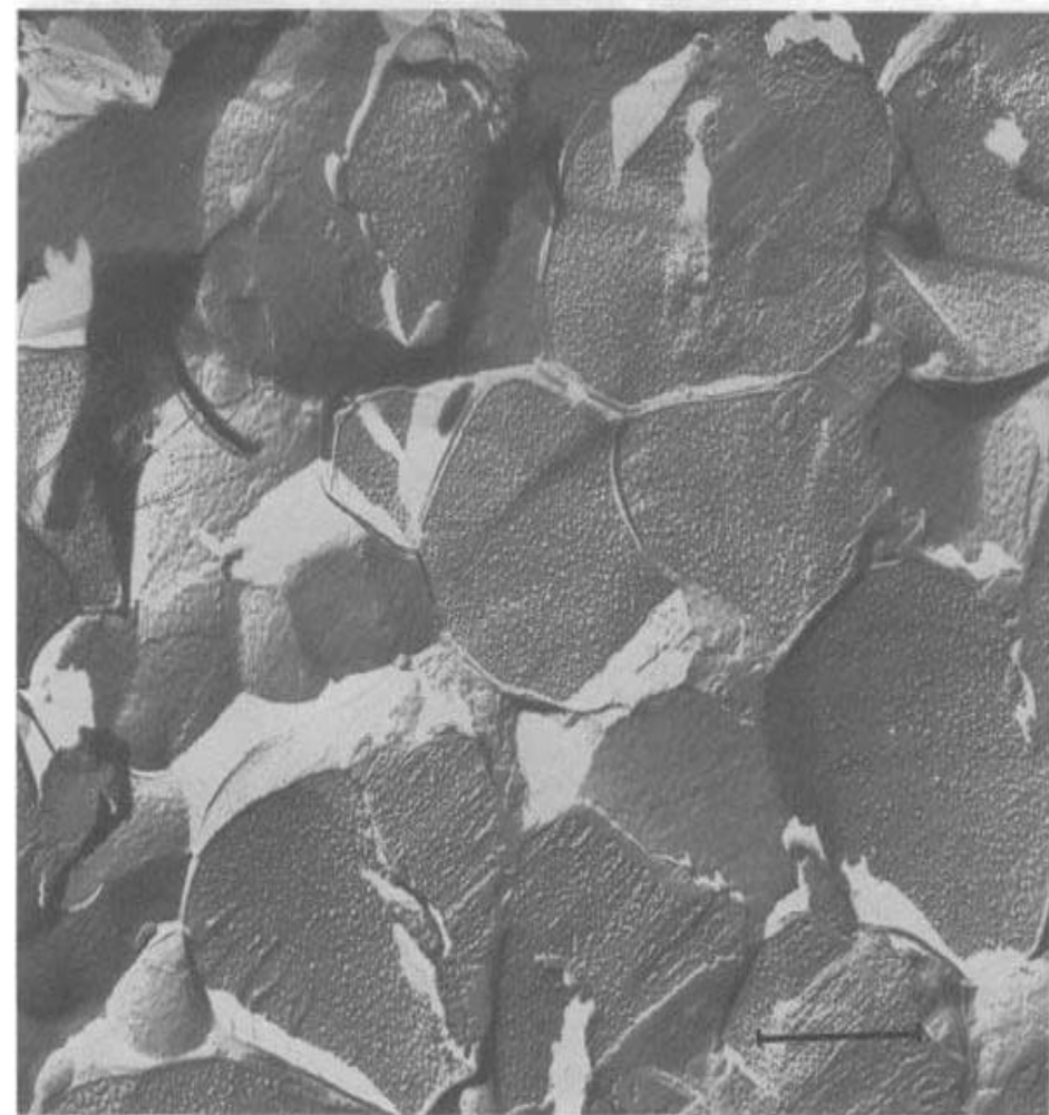
Fig. 10-24. Electron-micrograph of 5% TRS 10-410+3% isobutanol in 2% NaCl. 36,000 \times , bar = 1 \mu m.
